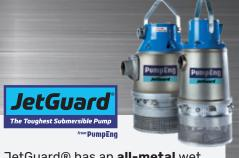
JetGuard® has an **all-metal** wet end with a high chrome impeller which makes it particularly suitable for harsh environments with Shotcrete poly fibre in the wastewater. The hydraulic water curtain guards against fibre entering the pump. JetGuard is suitable for underground mining, surface mining and general dewatering applications. It is available in 10kW and 20kW in 415V, 600V and 1,000V. (50 or 60 Hz)
